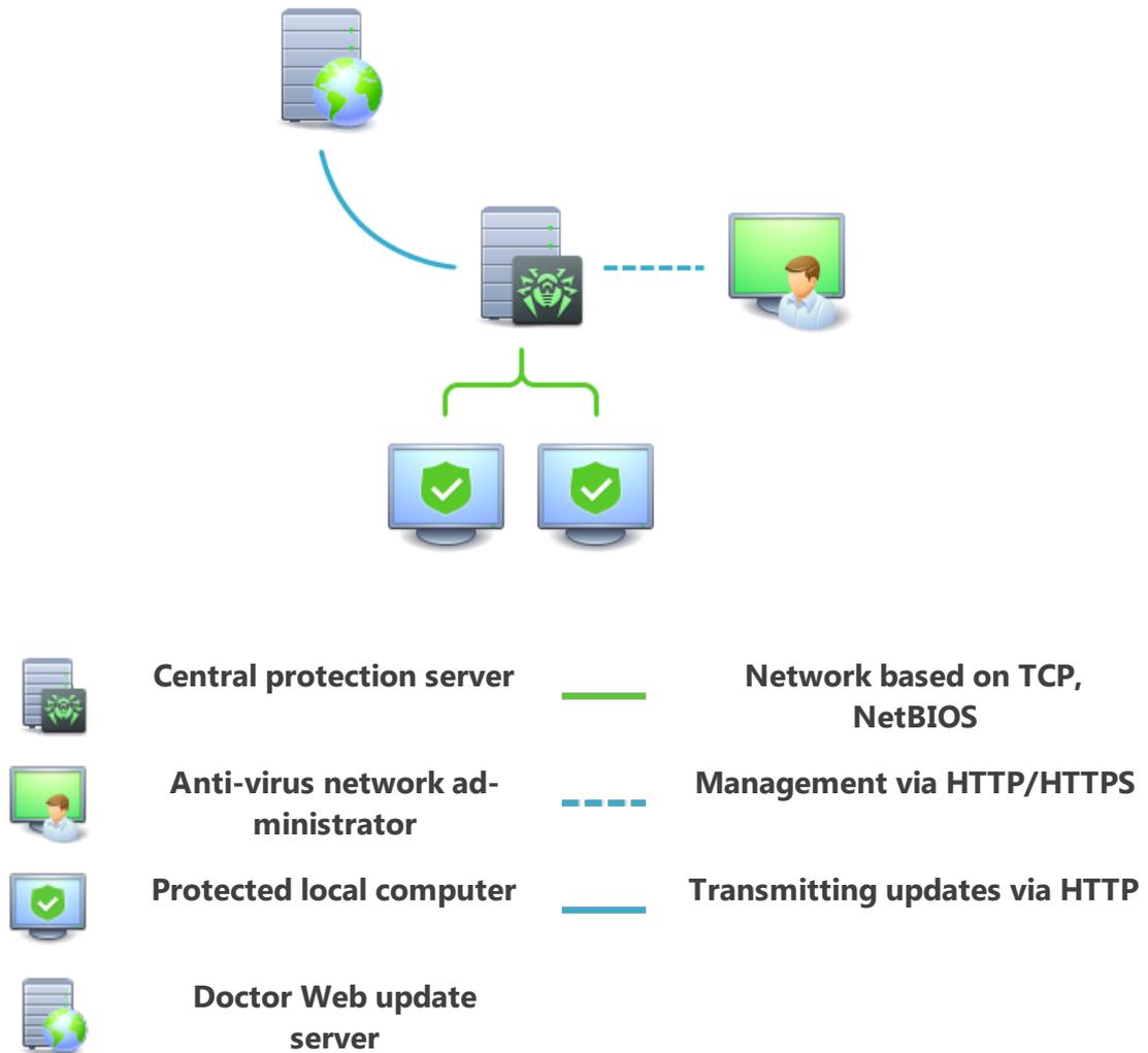
**Figure 17. Logical structure of anti-virus network.**
